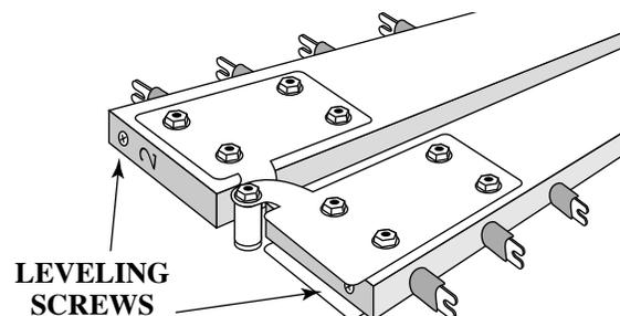
*Replace the rail and check it again. Reposition the bars as before.*
