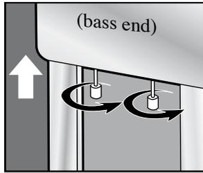
Turn the tuning knobs equally in the same direction until they elevate the bass resonator to approximately one inch below the arch in the lowest bass bar.
