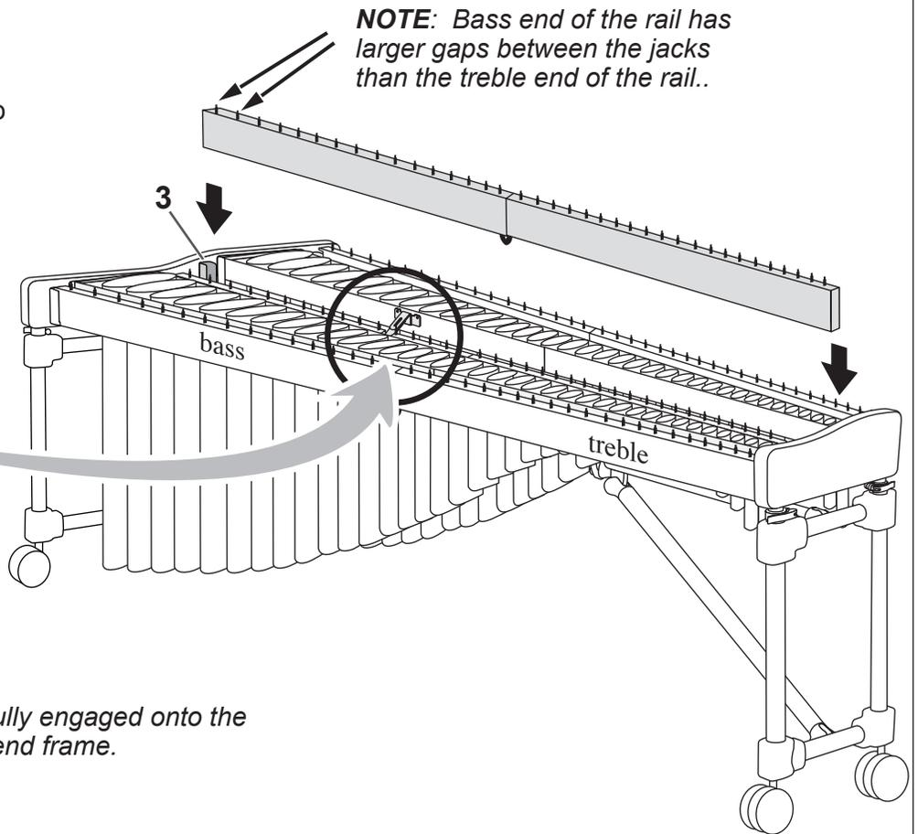
**NOTE:** Bass end of the rail has larger gaps between the jacks than the treble end of the rail..
