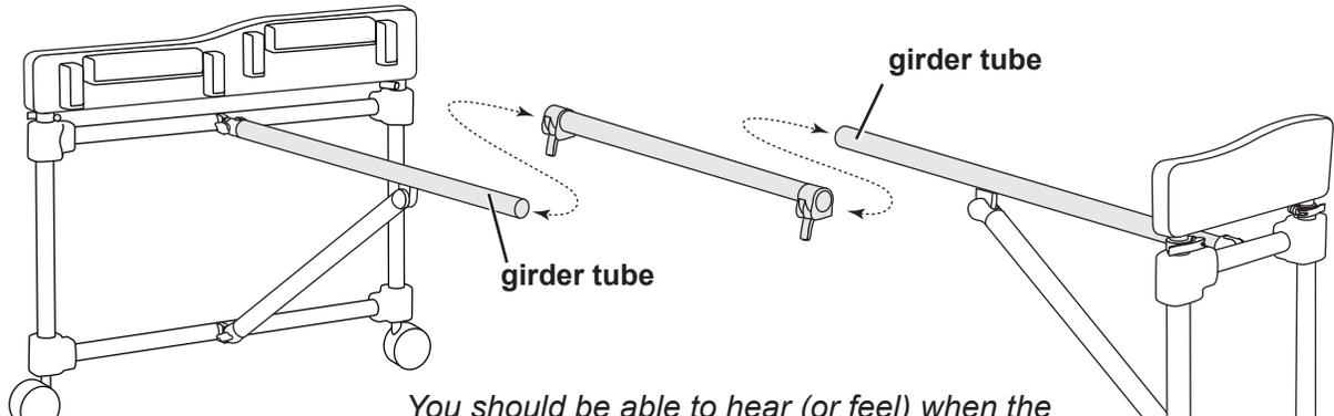
*You should be able to hear (or feel) when the two girder tubes touch inside the joiner-tube.*
