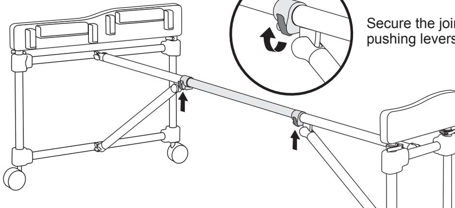
Secure the joiner-tube by pushing levers closed.
