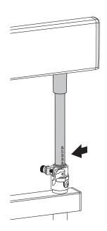
Locate the Izzy Height Adjustment™ clamp on the frame. b
