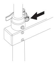
To increase clamping pressure turn wheel clockwise.
