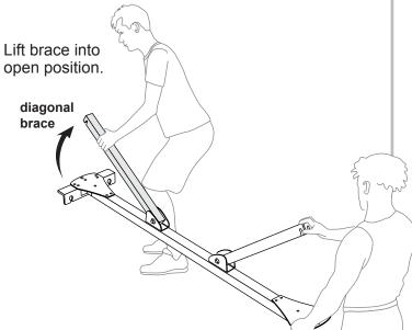
ATTACH DIAGONAL BRACE Lower slot onto clamp rod.
