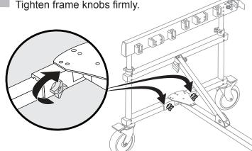
10 VERIFY CLAMPS AND KNOBS ARE SECURELY TIGHTENED
