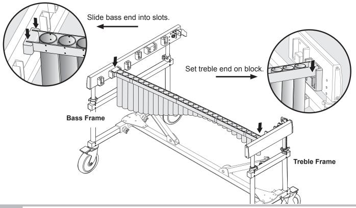
13 INSTALL ACCIDENTAL RESONATOR BANK Repeat steps for the second resonator bank.
