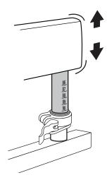
Gently lift or push down to raise or lower. Use gauges to ensure that both ends are always at the same height.
