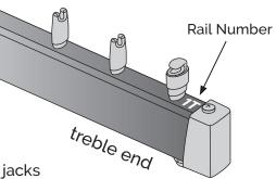
**NOTE**: Gaps between the rail jacks are wider on the bass end of rail.
