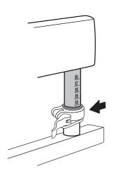
Locate the Izzy Height Adjustment™ clamp on the frame.
