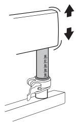
Gently lift or push down to raise or lower. Use gauges to ensure that both ends are always at the same height.
