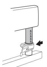
Locate the Izzy Height Adjustment™ clamp on the frame.
